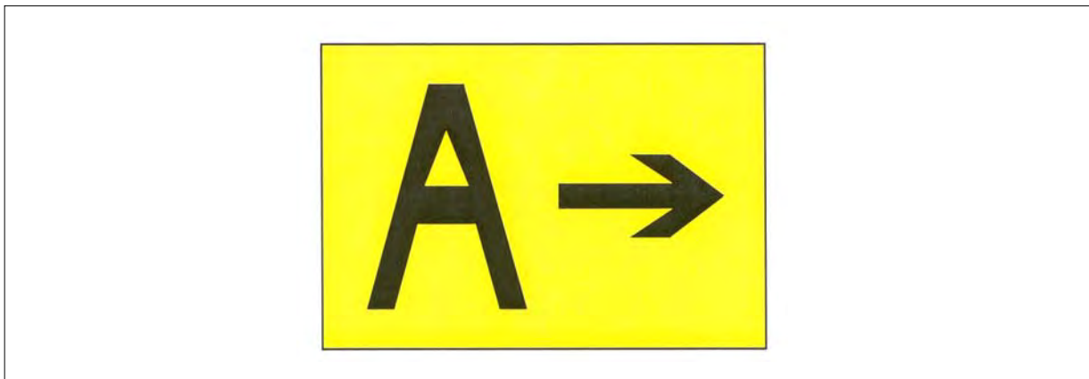
FIG AD 1.1-50 Direction Sign for Runway Exit
