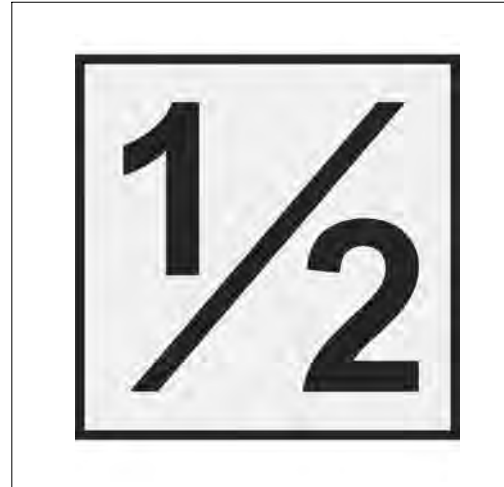
FIG ENR 5.7-1 Typical Runway Half-way Sign
