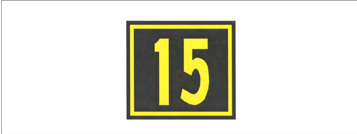
FIG AD 1.1-46 Runway Location Sign
