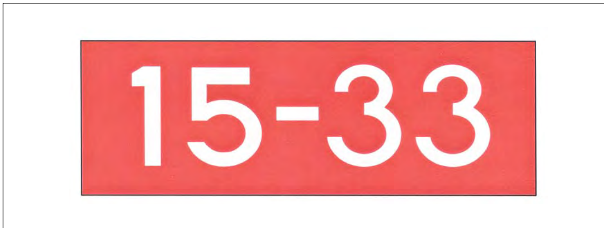
FIG AD 1.1-38 Runway Holding Position Sign
